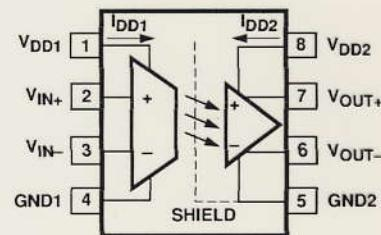
The product can also be used for general analog signal isolation applications requiring high accuracy, stability, and linearity under similarly severe noise conditions. For general applications, we recommend the HCPL-7840 (gain tolerance of  $\pm 5\%$ ). The HCPL-7840 utilizes sigma delta ( $\Sigma-\Delta$ ) analog-to-digital converter technology, chopper stabilized amplifiers, and a fully differential circuit topology fabricated using
